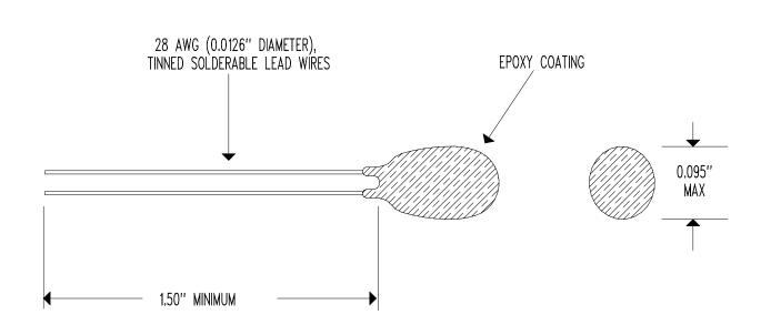
RESISTANCE @  $+25^{\circ}C = 30,000 \ \Omega \pm 10\%$  RESISTANCE/TEMPERATURE CURVE = "H" TEMPERATURE COEFFICIENT @  $+25^{\circ}C = -4.29\%$ /'C NOMINAL BETA " $\beta$ " (0 TO  $+50^{\circ}C$ ) = 3,810'K NOMINAL DISSIPATION CONSTANT = 1 mW/'C NOMINAL THERMAL TIME CONSTANT = 10 SECONDS MAXIMUM (STILL AIR) THERMAL TIME CONSTANT = 1 SECOND MAXIMUM (WELL STIRRED OIL) MAXIMUM TEMPERATURE RATING =  $+150^{\circ}C$
