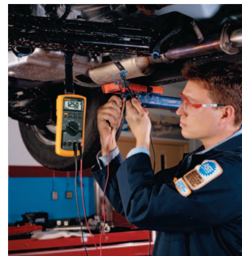
Powerful magnet holds meter to most steel surfaces
