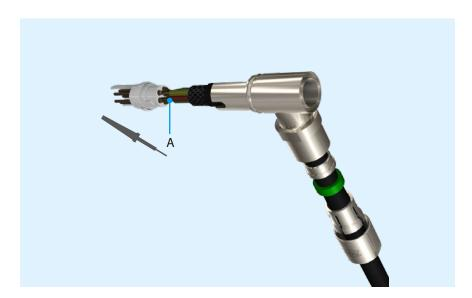
5. Bend cable shield outwards, place half-shells and right-angled part over insulator.
