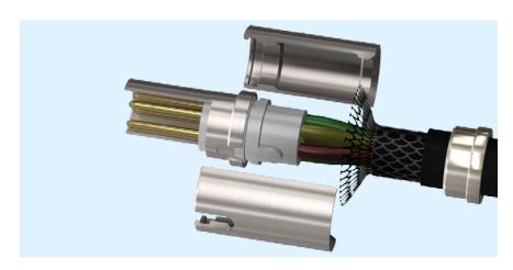
6. Slide the EMI ring and the cable collet against the half-shells and clamp the shield against it.
