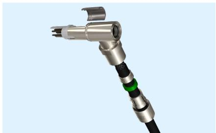
6. Slide EMI ring, sealing, washer and cable collet against the right-angled part, and clamp shield between EMI ring and right-angled part. If necessary, secure thread (B) with adhesive (see page 19). Screw back nut on the assembled plug, counterhold by means of the spanner flat (C) and hold against with ODU spanner wrench.
