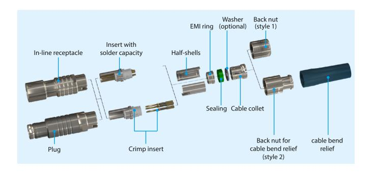
1. Slide cable bend relief, back nut, cable collet, washer, sealing and EMI ring over the cable.
