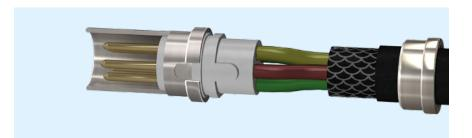
5. Bend cable shield outwards, assemble half shells.
