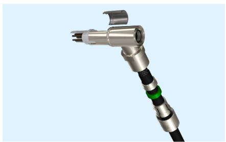
6. Slide EMI ring, sealing, washer and cable collet against the right-angled part, and clamp shield between EMI ring and right-angled part. If necessary, secure thread (B) with adhesive (see page 19). Screw the back nut, counterhold by means of the spanner flat (C) and tighten it with ODU spanner wrench.
