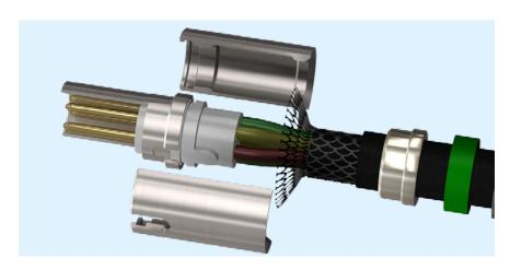
6. Slide the EMI ring, sealing, washer and the cable collet against the half-shells and clamp the shield against it.
