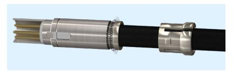
7. Put the assembled cable considering the guidings (C) in the connector housing. If necessary, secure thread (B) with adhesive (see page 18).
