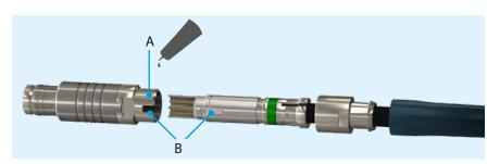
8. Screw back nut on the assembled plug, counterhold by means of the spanner flat (C) and hold against with ODU spanner wrench.
