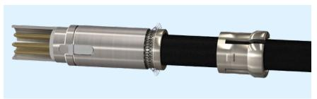
7. Put the assembled cable considering the guidings (B) in the connector housing. If necessary, secure thread (A) with adhesive (see page 18).
