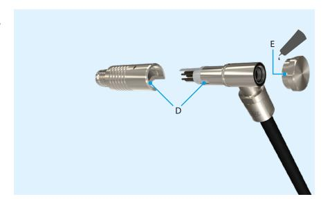
8. Mount back screw on the assembled plug and counterhold by means of the spanner flat (F) with ODU spanner wrench.
