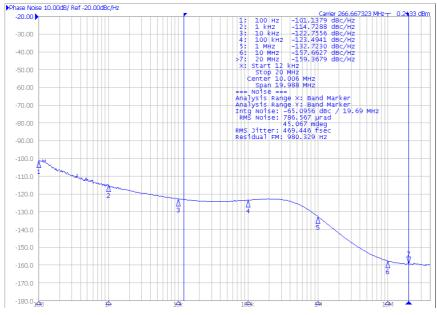
Figure 3. Typical Phase Noise Plot
