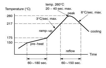
Figure 5. Recommended Reflow Soldering Profile
