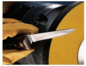
Buff and Polish Unitized Wheels are a unitized constructed, non-abrasive carrier for compounds used for polishing flat and symmetrical contoured surfaces. They can often replace felt or leather wheels, as they hold more compound with even distribution allowing for faster cut and less frequent compound application.
