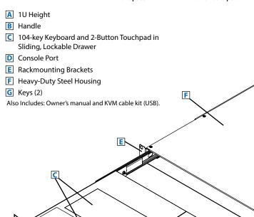
The SRSHELFKBD SmartRack® 1U Rack-Mount Keyboard is a full 104-key keyboard and two-button touchpad designed for mounting in an EIA-standard 19-inch rack. It can be mounted in a 2- or 4- post rack. Tripp Lite's B019-000 bracket (sold separately) is required for two-post mounting. It's ideal for use with KVM switches and servers that don't include a keyboard.
