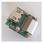
A set of connectors to extend the Raspberry Pi camera cable with a standard HDMI cable.
