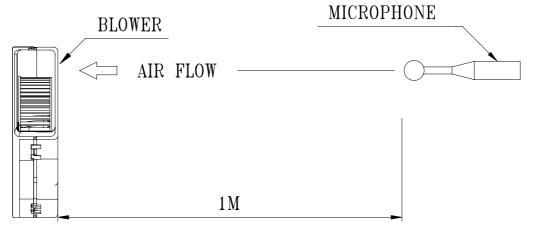
NOISE IS MEASURED AT RATED VOLTAGE IN FREE AIR IN ANECHOIC CHAMBER WITH B & K SOUND LEVEL METER WITH MICROPHONE AT A DISTANCE OF ONE METER FROM THE FAN INTAKE.
