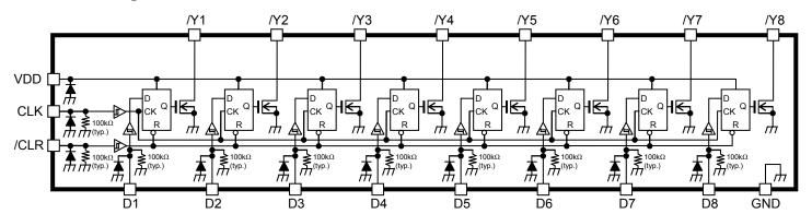
Equivalent circuit may be omitted or simplified for explanatory purpose.
