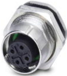
Bus system flush-type socket, ETHERNET and PROFINET, 4-pos., M12 SPEEDCON, shielded, D-coded, rear/screw mounting with Pg9 thread, with straight solder connection
