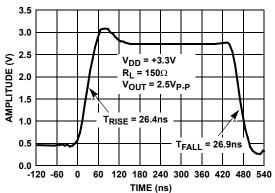
FIGURE 11. LARGE SIGNAL STEP RESPONSE
