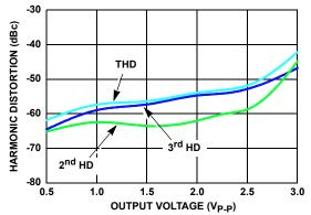
FIGURE 16. HARMONIC DISTORTION vs OUTPUT VOLTAGE
