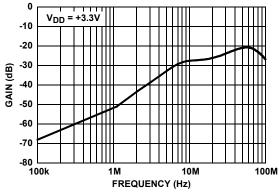
FIGURE 6. PSRR vs FREQUENCY
