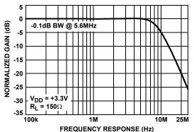
FIGURE 1. GAIN vs FREQUENCY -0.1dB
