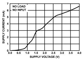
FIGURE 10. SUPPLY CURRENT vs SUPPLY VOLTAGE
