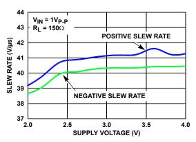
FIGURE 19. SLEW RATE vs SUPPLY VOLTAGE
