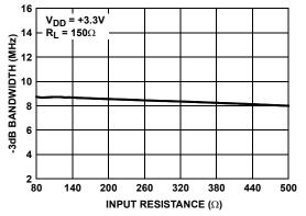
FIGURE 18. -3dB BANDWIDTH vs INPUT RESISTANCE
