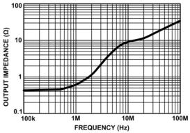
FIGURE 7. OUTPUT IMPEDANCE vs FREQUENCY
