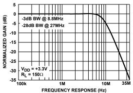
FIGURE 2. GAIN vs FREQUENCY -3dB POINT
