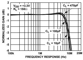
FIGURE 3. GAIN vs FREQUENCY FOR VARIOUS  $C_{\mbox{\scriptsize LOAD}}$
