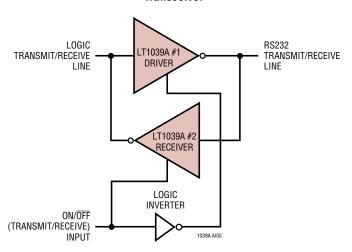
The shutdown mode also drops all supply currents ( $V_{CC}$ ,  $V^+$ ,  $V^-$ ) to zero for power conscious systems.
