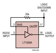
It can also be used to make an RS232 compatible shutdown control line. Driving the BIAS pin low through a resistance of 24k to 30k keeps the receiver active. Do not drive the BIAS pin directly from a logic output without the series resistor. An unused BIAS pin should be left open.
