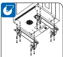
For applications requiring extra mobility, an optional caster kit (Model: CSHANDLEKIT) contains two swivel/locking casters and two swivel-only casters that attaches to the bottom of a charging station unit.
