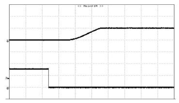
**Figure 14:** Turn on Using Remote On/Off with external capacitors (Co=3000µF), 5.0V/5A out (resistive load) (5mS/div) Top trace: Vout, 5V/div; Bottom trace: On/Off, 2V/div
