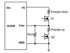
Figure 26: Circuit configuration for output voltage margining
