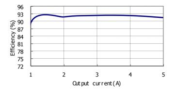
Figure 1: Converter efficiency vs. output current (12V in, 5V output voltage)
