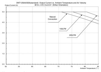
Figure 29: Output current vs. ambient temperature and air velocity @ Vin=12V, Vo=5.0V (Either Orientation)
