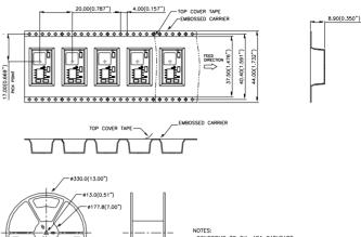
NOTES: CONFORMS TO ELA-481 SATNDARD MODULES ARE SHMPPED IN QUANTITIES OF 100 PER REEL. ALL DIMENSIONS ARE IN MULLIMETERS AND (INCHES) TOLERANCES: X.Xmm±0.5mm(X.XXX in.±0.02 in.) X.XXmm±0.5mm(X.XXX in.±0.01 in.)
