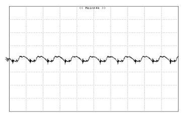
Figure 9: Output ripple & noise at 12Vin, 2.5V/5A out pk-pk :31.25mV, rms :7.38mV (50mv/div,2uS/div )
