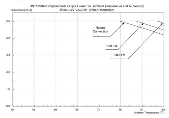
Figure 30: Output current vs. ambient temperature and air velocity @ Vin=12V, Vo=3.3V (Either Orientation)
