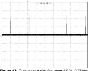
Figure 17: Output short circuit current 12Vin, 0.75Vout (10A/div, 50mS/div)
