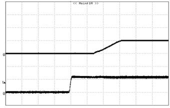
*Figure 13: Turn on Using Input On/Off with external capacitors (Co=3000µF), 5.0V/5Aout (resistive load) (5mS/div)*
