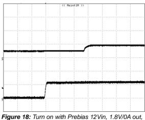
*Figure 18:* Turn on with Prebias 12 Vin, 1.8V/0A ou Vbias =1.0Vdc. (5mS/div) Top trace: Vout, 2V/div; Bottom trace: Vin, 10V/div
