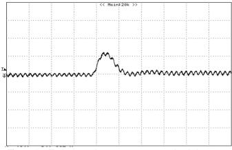
**Figure 15:** Typical transient response to step load change at 2.5A/µS from 100% to 50% of lo, max at 12Vin, 5.0V out (Cout= 1uF ceramic+ 10µF Tantalum)(200mV/div, 10uS/div)
