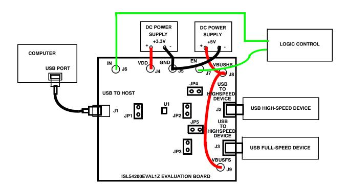
Note: Disconnect the +5V power supply connected to J8 and J9 when powering through Host Controller Bus.
