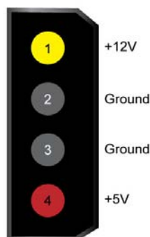
Figure 4-3 ATX Power Connector
