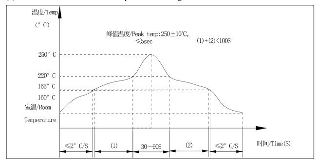
回流焊技术要求/Technical requirements for reflow
