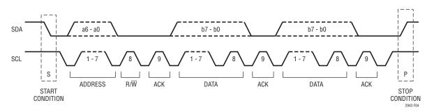
Figure 4. Data Transfer Over I<sup>2</sup>C or SMBus
