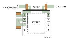
Figure 12. Kelvin Connection on Sense Resistor
