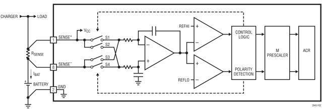
Figure 2. Coulomb Counter Section of the LTC2943
