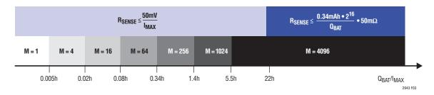
Figure 3. Choice of Sense Resistor and Prescaler as Function of Battery Capacity and Maximum Current
