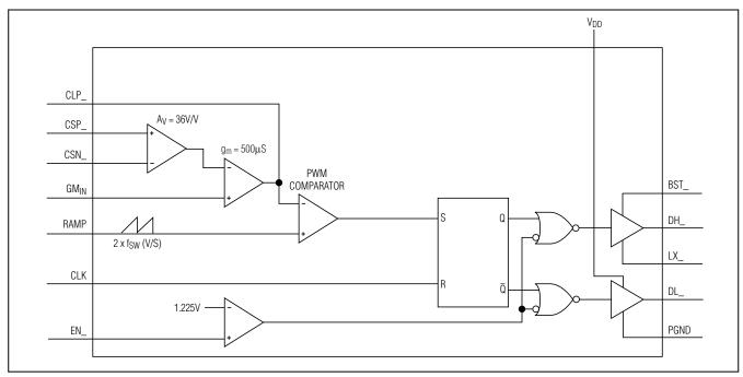
Figure 3. Current Comparator and MOSFET Driver Logic
