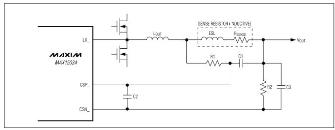
Figure 10. Inductive Sense Resistor
