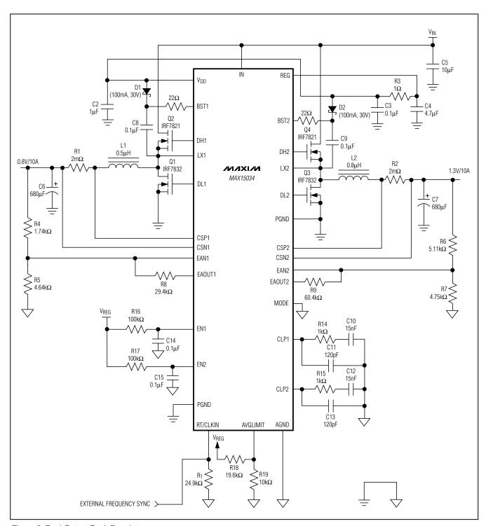
Figure 6. Dual-Output Buck Regulator
