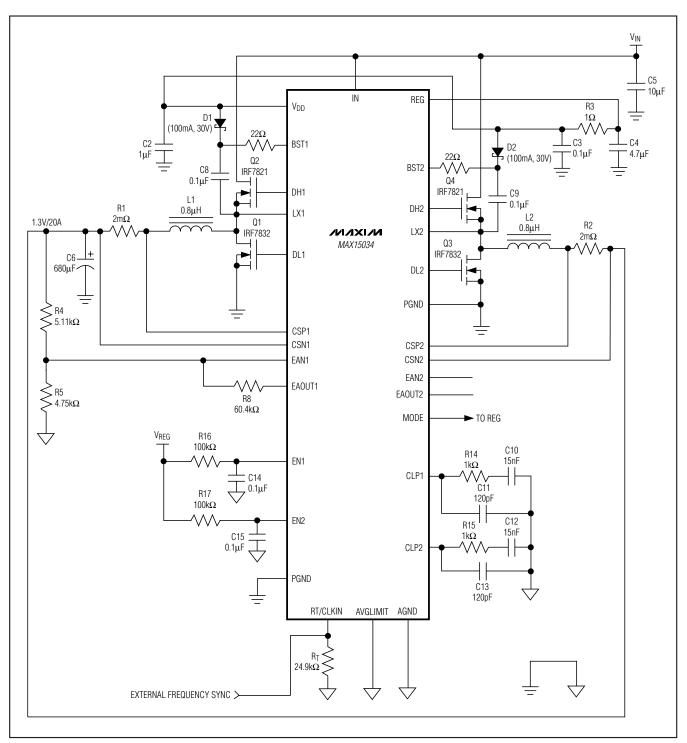
Figure 7. Dual-Phase, Single-Output Buck Regulator
