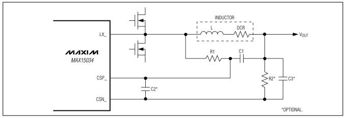
Figure 9. Lossless Inductor Sense
