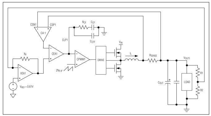
Figure 2. Current and Voltage Loops
