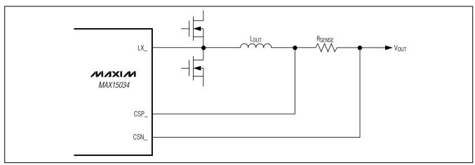
Figure 8. Noninductive Resistive Sense
