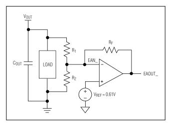
Figure 4. Voltage Error Amplifier
